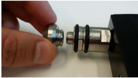
1. Align bezels of adaptor to corresponding notches on probe tip
