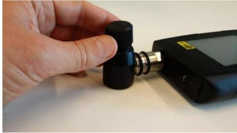
Screw the cap on and start the measurement.
