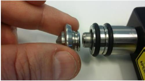
1. Align bezels of adaptor to corresponding notches on the probe tip.
