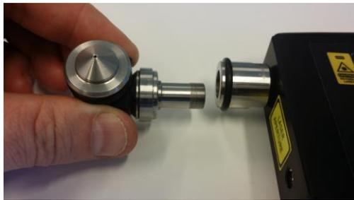
Attach the angled probe tip by gently inserting the threaded part and screw it in place by hand. Use the wrenches to tighten. Make sure that the tip is securely fastened, but do not overtighten.
