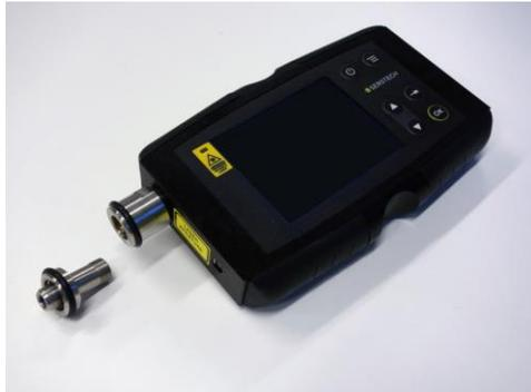
Hold the wrench next to the instruments main body still and turn the wrench on the probe tip counterclockwise to remove it.
