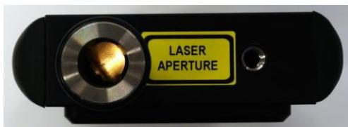
**NOTE:** Make sure not to damage the invisible laser shutter when mounting the angled probe tip. The invisible laser shutter prevents any accidental exposure to the collimated laser beam.
