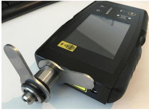
To mount the angled probe tip first remove the current probe tip from the instrument. Use two specially designed wrenches supplied with the instrument.
