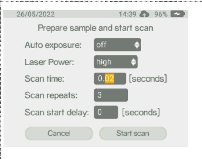
If Auto exposure is OFF, the Scan time must be set; it can have any value between 0.02 s and 65.5 s. Set number of scan repeats to create the reference spectrum; the minimum is 3.
