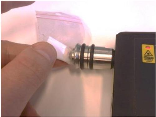
With the point and shoot adaptor the measurements can be made e.g. through transparent plastic bags by gently pressing the adaptor against the bag.
