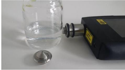
Measure without an adaptor if your container is 1.5- 4.0 mm thick. Place the container flush to the instrument probe tip and start the measurement.
