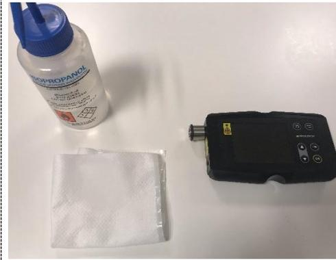
The standard way to clean the instrument is to moist with Isopropanol a lint-free cloth.
