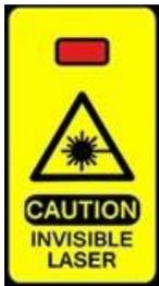
On the front side of the Indicator there is a clearly visible **laser warning label** with a red indicator LED that is lit when the invisible laser is operating.
