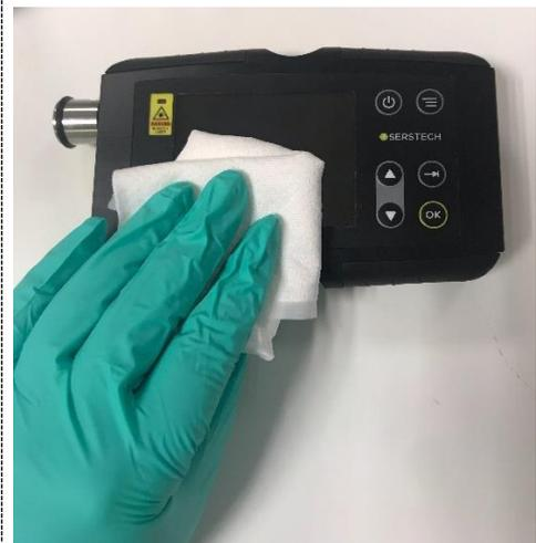
Before starting cleaning the instrument, make sure to turn off the device and remove all accessories from it.
