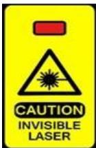
**WARNING:** Keep the sample pressed against the adaptor until the red diode, indicating invisible laser activity, is turned off.
