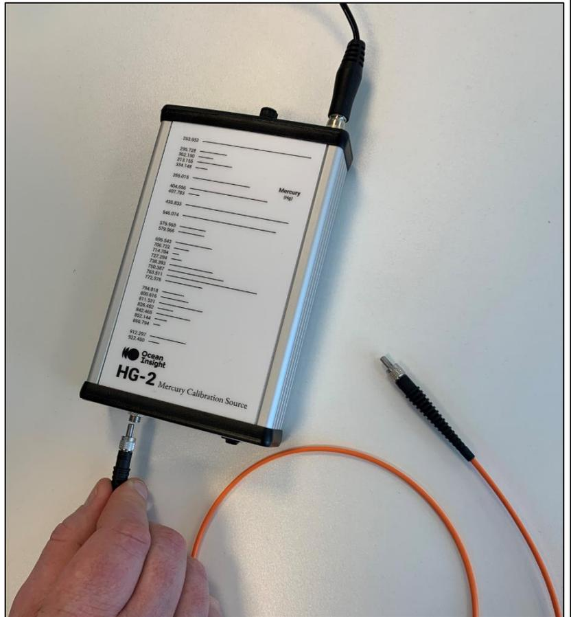
Attach the fiber adapter to the optical fiber cable.
