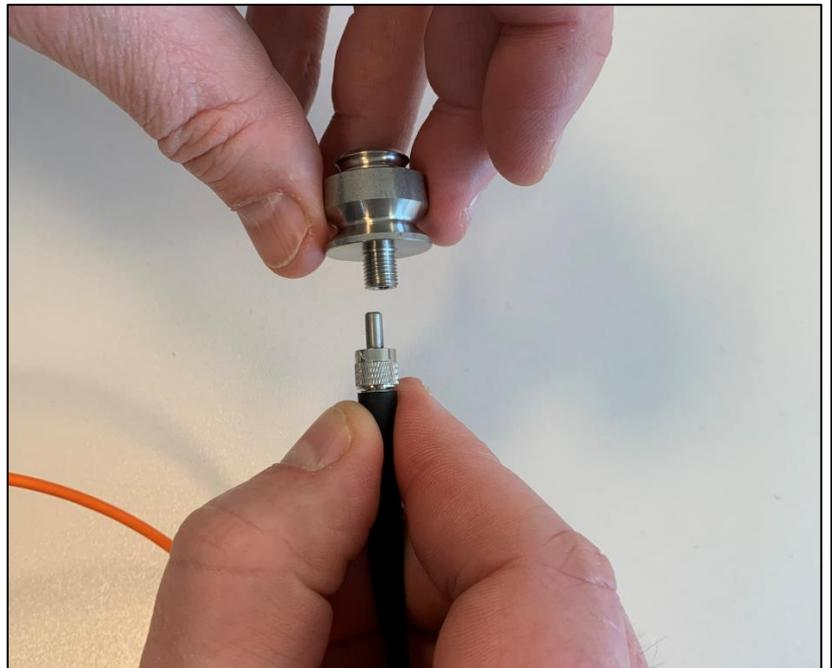
Put the adapter on the indicator's probe.
