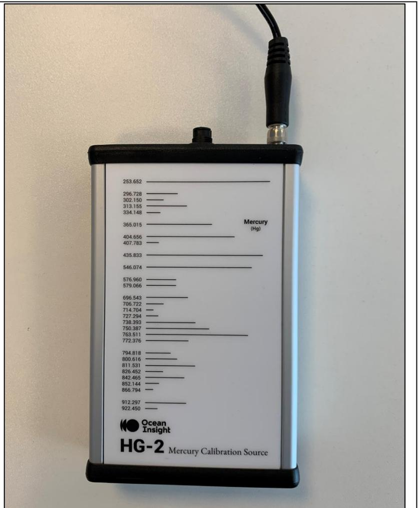
Connect the optical fiber by attaching it to the lamp fiber output and turn it ON. (Leave it ON for about 2 minutes before running the test).
